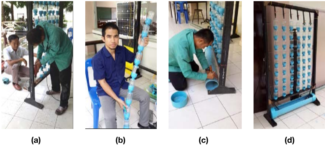
Figure 3 Steps of making the KUS-58 Hydroponic Kit (a) drilling the frame (b) connecting 9 plastic bottles vertically (c) installing PVC tube for soluble nutrients and air pump (d) the KUS-58 Hydroponic Kit
