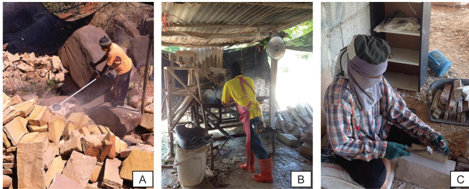
Fig. 2 Tasks of sandstone worker. (A) Stone cutting worker at site with a grass cutter like stone cutter. (B) Stone cutting at home with a stone cutter. (C) Stone cut and decorated with hand chisel.
