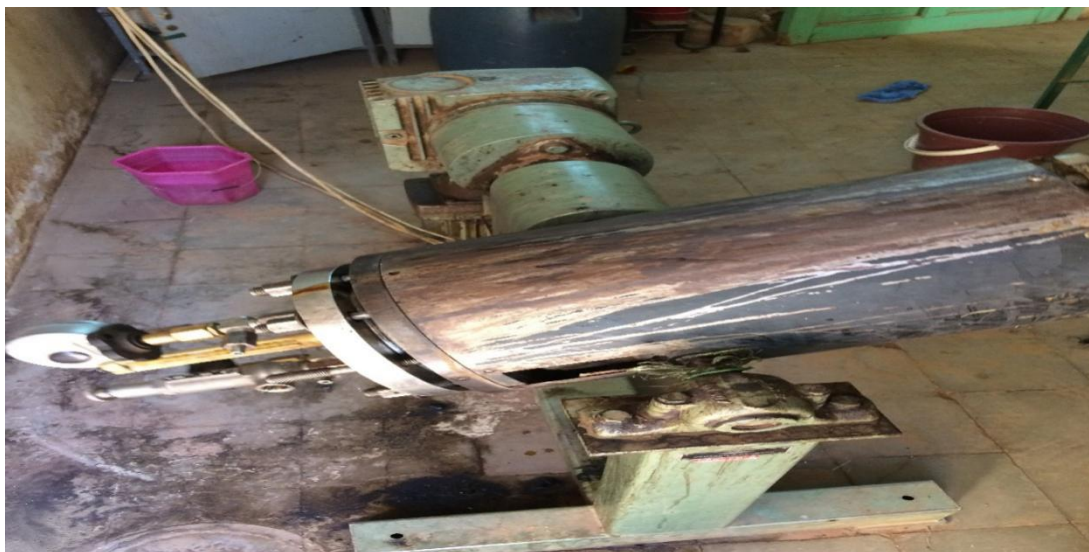
Figure 2 The digester used during pulping of Citrus limon with soda, Soda-AQ, AS-AQ and ASAM methods.
