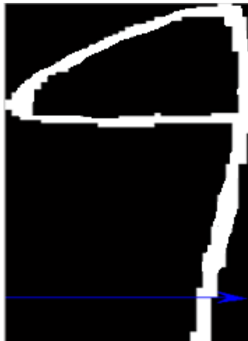
Figure 8 View of the scanned Arabic object number 9 to count the number of flips.
