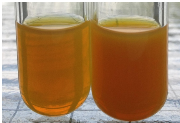
Figure 2 Macroscopic appearance of 0.5 % CoQ 10 -loaded usNLC (left) and 5.0 % CoQ 10 -loaded usNLC (right).
