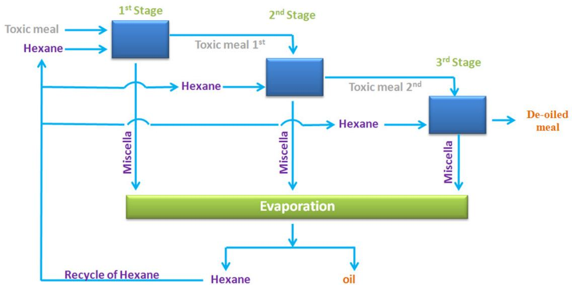
Figure 2 Schematic procedure of the oil extraction.
