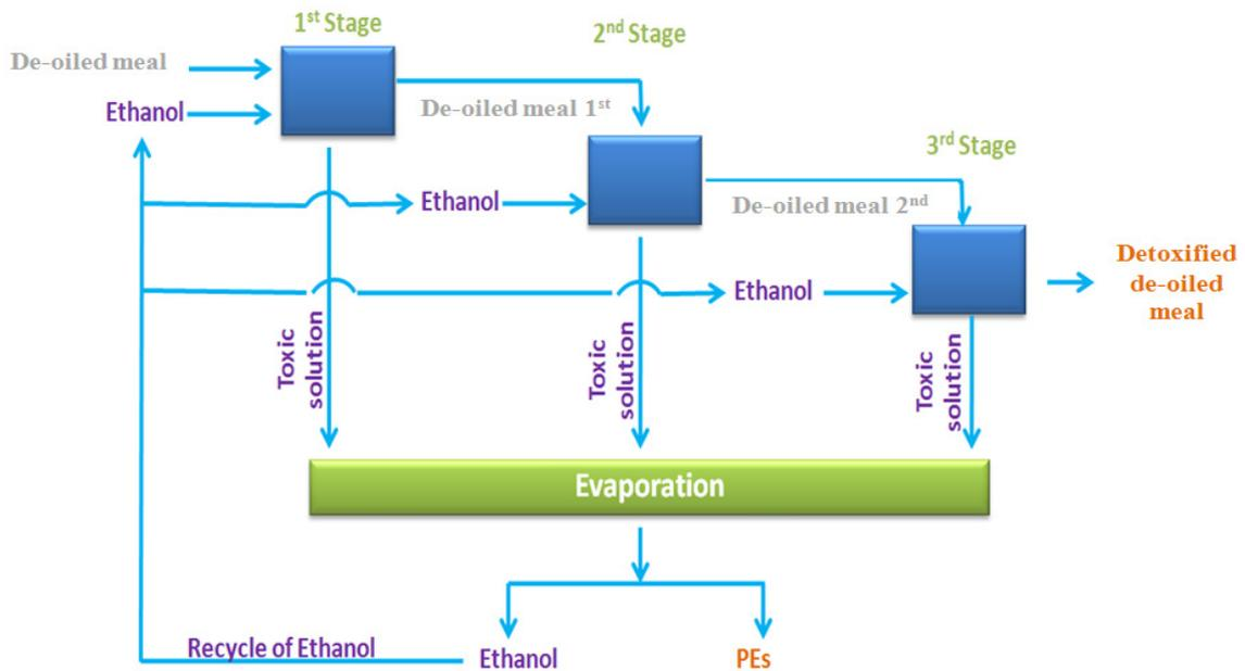
Figure 3 Schematic procedure of the PEs extraction.
