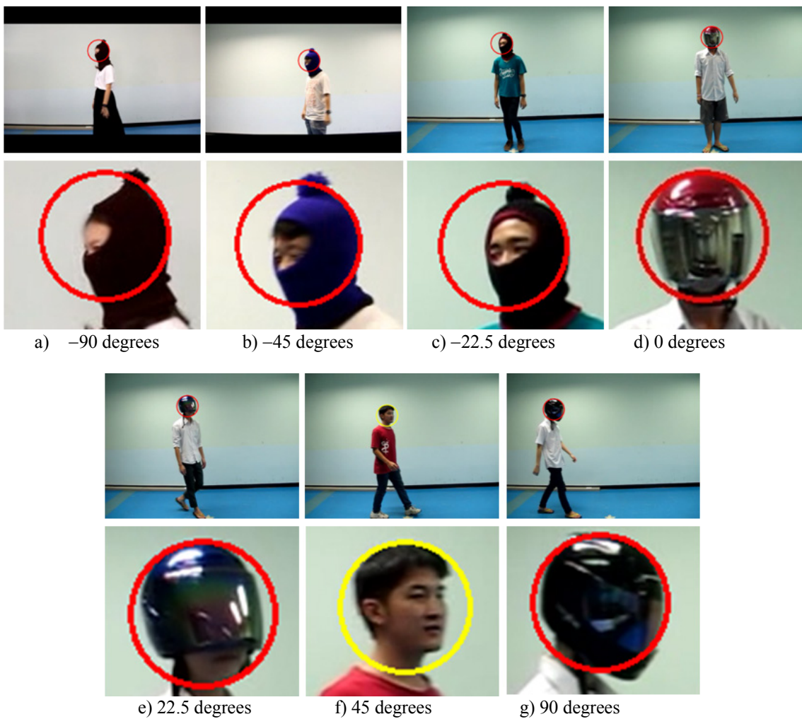
Figure 7 Correct results of occluded and non-occluded face detection.
