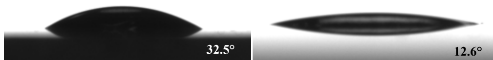
Figure 9 The image of water droplet contact angles after 0 and 60 min UV irradiation of TiO 2 /5SnO 2 thin films.
