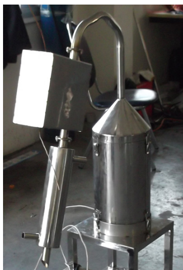
Figure 4 The small scale essential oil refiner with CEOHP.
