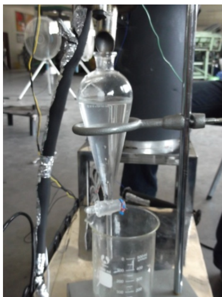
Figure 6 The separatory funnel containing the essential oil.
