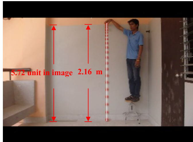
Figure 1 Composite image from the free falling sequences.
