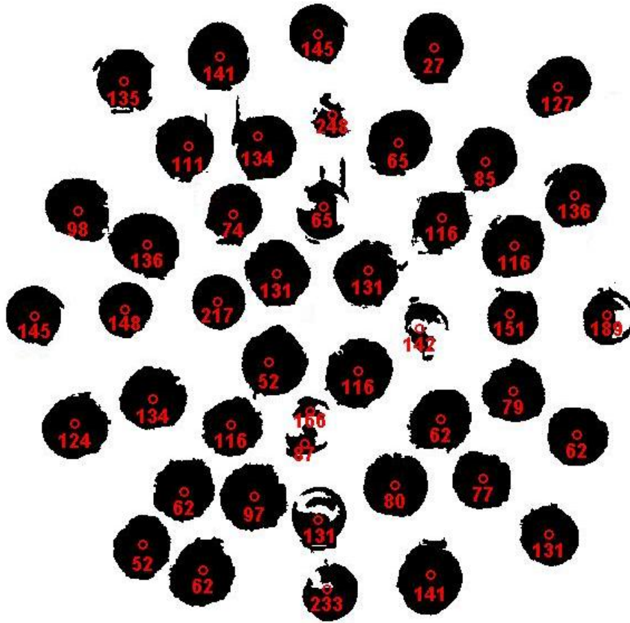
Figure 5 The result of using the routines to identify the center of all LEDs, measure and display the brightness levels.
