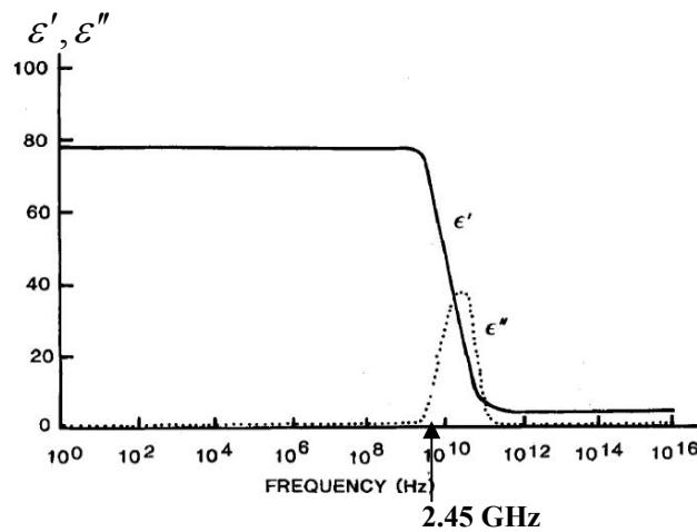
**Figure 1** Dependence of  $\epsilon'$  and  $\epsilon''$  on microwave frequency in liquid water at 25 °C [5].
