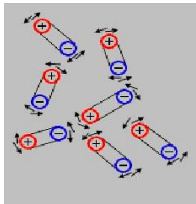
**Figure 2** Model of rotation of dipoles in dielectric materials caused by alternating electric field component of the microwave [5].
