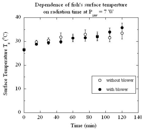
**Figure 10** Dependence of  $T_s$  on radiation time at  $P_{\mu\text{w}} = 7 \text{ W}$  when the blower is on or off.
