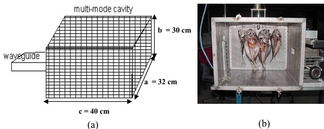
**Figure 8** (a) Schematic diagram and (b) picture of multi-mode cavity for microwave excitation at 2.45 GHz.
