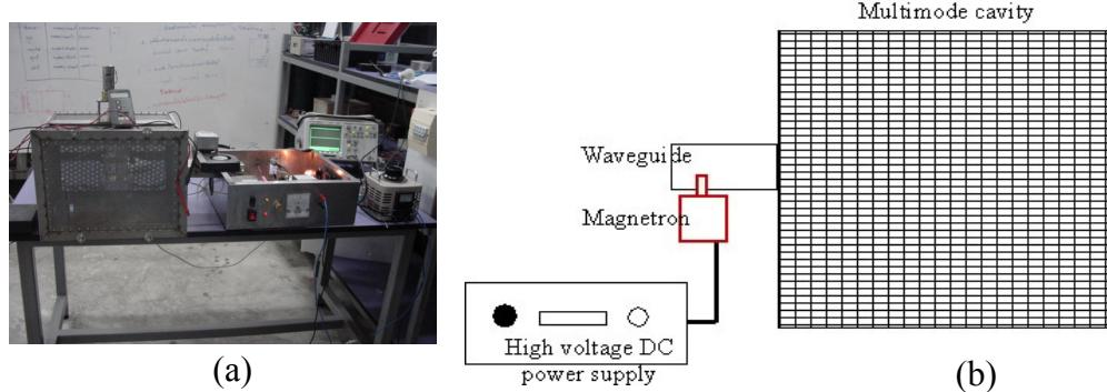
**Figure 3** (a) Picture of experimental setup and (b) schematic diagram of experimental setup.
