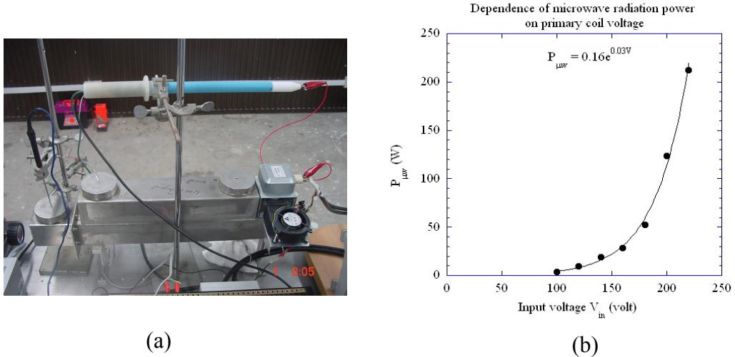
**Figure 6** (a) Experimental setup for microwave power calibration, (b) dependence of microwave power  $P_{\mu w}$  on input voltage  $V_{in}$ .
