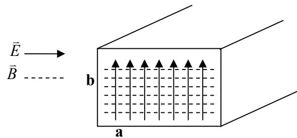
**Figure 7** Cross-section of the rectangular waveguide. Dashed and solid lines represent electric and magnetic microwave fields respectively.
