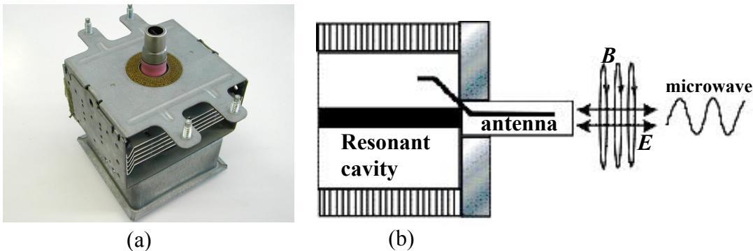
**Figure 4** (a) Picture of a commercial magnetron and (b) schematic diagram of a magnetron.
