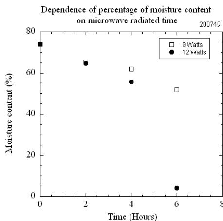
**Figure 11** Dependence of percentage of moisture content on microwave power after radiating for 6 h.
