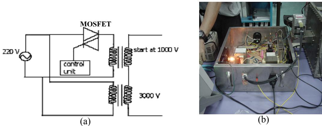
**Figure 5** (a) Schematic circuit of High-Voltage Power Supply and (b) picture of HV power supply.
