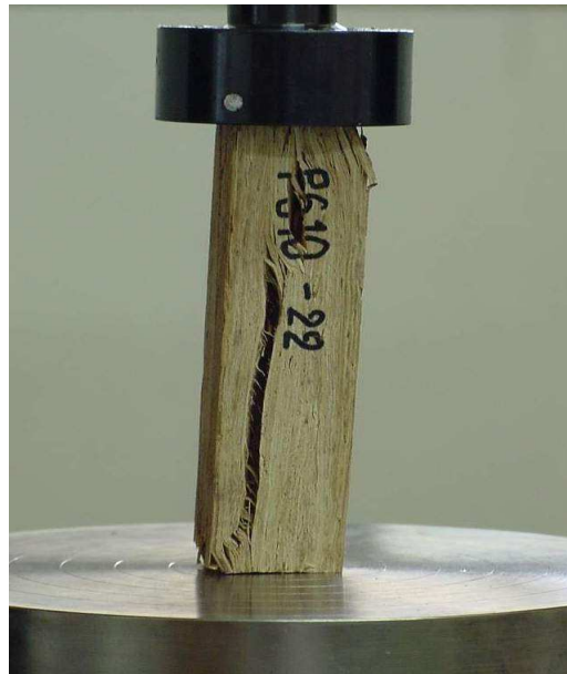
Figure 10. Tension perpendicular-to-grain failure in a specimen under compression parallel-to-grain test.
