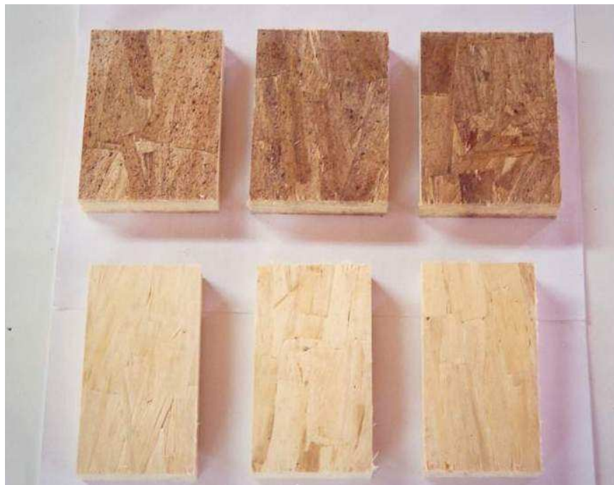
Figure 4. Oriented strand lumber made from PF resin (upper) and pMDI resin (lower).
