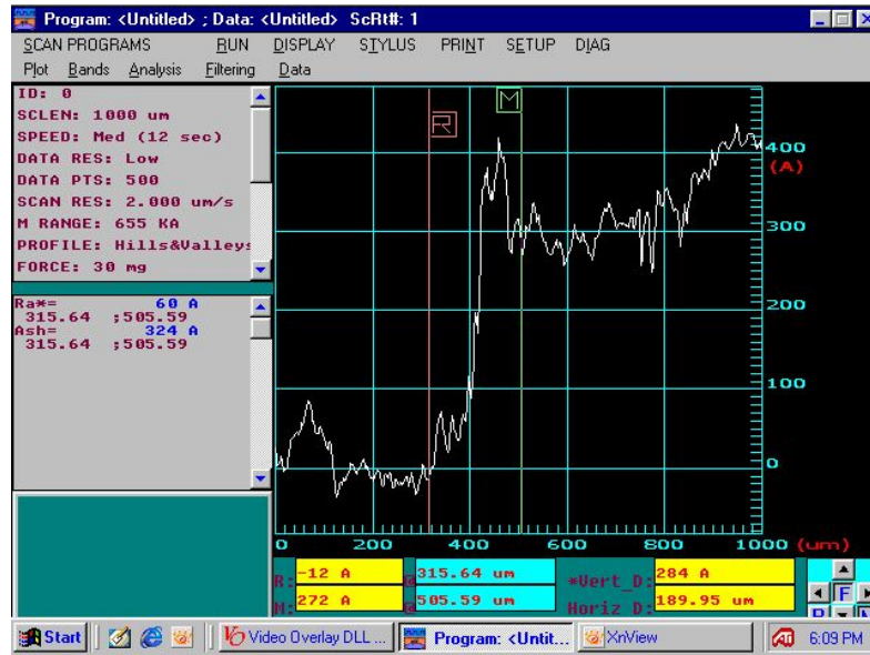
Figure 4. Thickness of a cobalt film indicated by stylus method profilometry.
