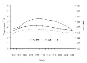
**Fig. 10.** Air flow temperature and power from natural daylight.
