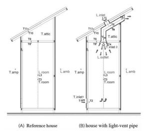
**Fig. 2.** The measuring positions of temperatures, illuminance and air velocity.
