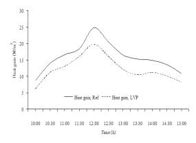
Fig. 15. Hourly variation of ceiling heat gain.
