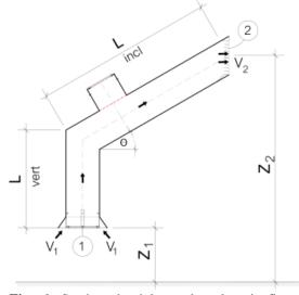
Fig. 6. Section the inlet and outlet air flow model.
