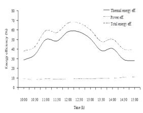
**Fig. 12.** Thermal energy, power energy from daylight and total energy efficiency of LVP.
