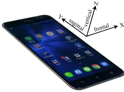
Fig. 2. Inclination directions relative to tri-axial accelerometers in a smartphone.
