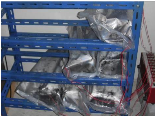
7(b) curing by wet clothes and plastic sheets until the age of 7 days
