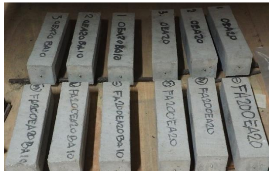
4a) Specimens for free expansion/shrinkage test
