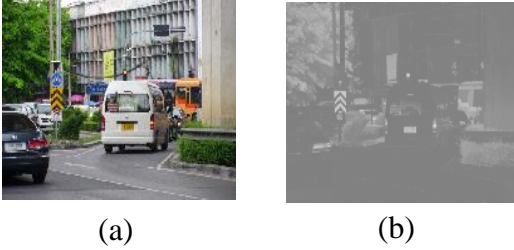
Fig.5. Traffic light extraction result. (a) Input image, and (b) ab* image.
