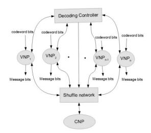
**Fig.2.** The architecture of flexible LDPC decoder.
