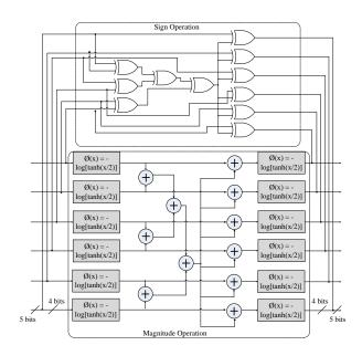
Fig.3. The architecture of CNP.
