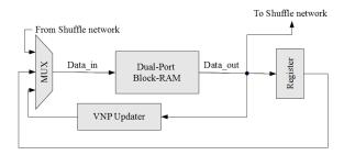
(c) Register insertion in all VNPs of Scheme
