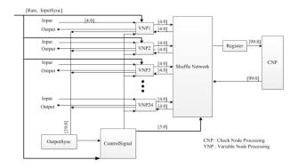
(a) Overall architecture of Scheme 1: a stage of register is added between shuffle network and CNP
