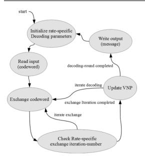
Fig.7. Finite State Machine of LDPC Decoder.
