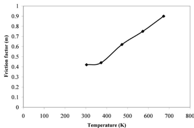
**Fig. 6.** The plot of friction factor for Al-5Zn-1Mg alloy with temperature using MoS<sub>2</sub> lubricant.
