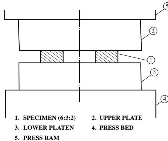
**Fig. 1.** Schematic set up of ring compression test [13].
