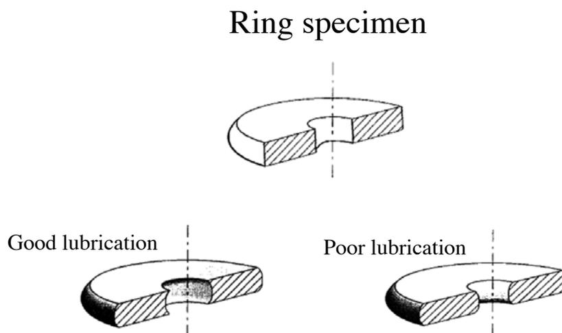
**Fig. 2.** Ring compression: (a) before compression, (b) after compression with low friction and (c) after compression with high friction.[7].
