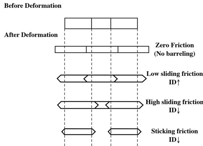
Fig. 4. Types of ring deformations after compression [9, 10]
