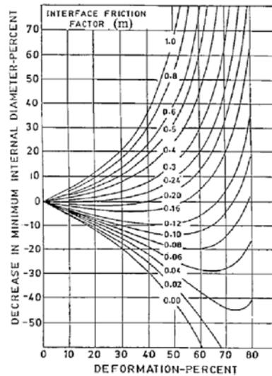
Fig. 3. Calibration chart to determine friction factor (m) [8].
