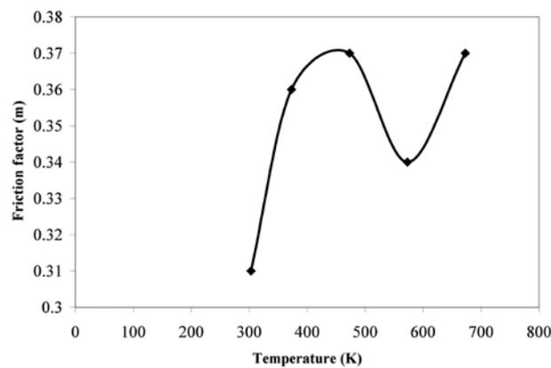
**Fig. 5.** The plot of friction factor for Al-5Zn-1Mg alloy with temperature using graphite lubricant.
