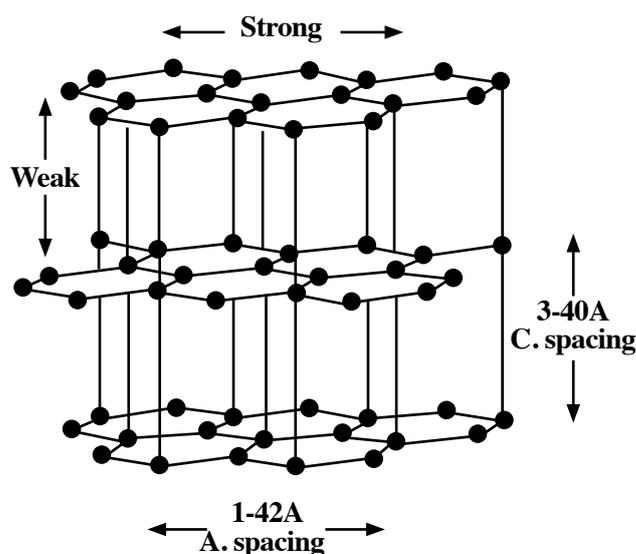
**Fig. 7.** Structure of graphite. The individual sheets consist of closely packed atoms, separated by a relatively large distance from neighbouring sheets. [15].
