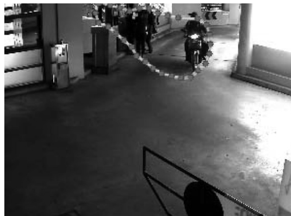
Fig. 4. Converged contour in the case of multiple objects.
