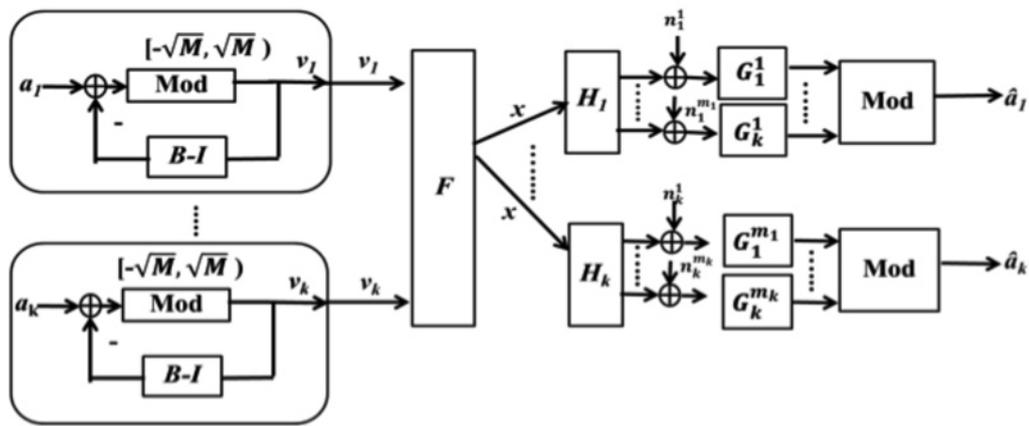
Fig. 2. System model of downlink MU-MIMO THP.
