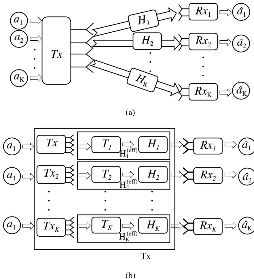
**Fig. 1.** System model of Downlink MU-MIMO system (a) the overall system, (b) the effective system with block diagonalization.
