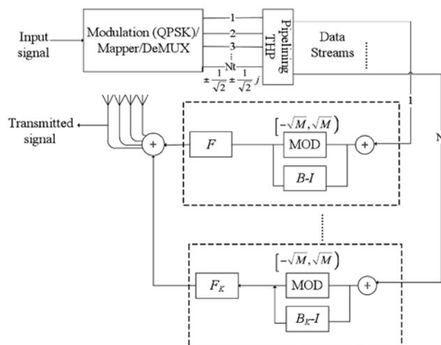
**Fig. 3.** Concatenated PIPTHP ( C-PIPTHP) for Downlink MU-MIMO at Transmitter (Tx).
