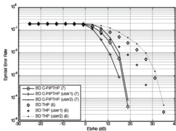
**Fig. 9.** Performance comparison for SER of BD C-PIPTHP and BD-THP for one user. BD C-PIPTHP (7) for user 1 gives the best SER performance of all downlink MU-MIMO THP-based schemes.
