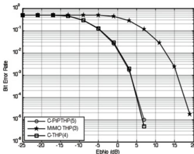
**Fig. 5.** BER performance for downlink MIMO THP-based schemes. The new concatenated systems, C-THP (4) and C-PIPTHP (5), give better BER than the traditional MIMO THP (3). In C-PIPTHP (5), although its performance is comparable to C-THP (4), pipelining also improves the processing time as shown in Table 2.
