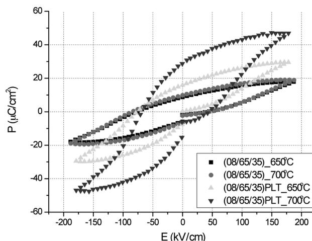
**Fig. 4.** Ferroelectric hysteresis for the PLZT films without and a with seeding layer annealed at 650-700°C.
