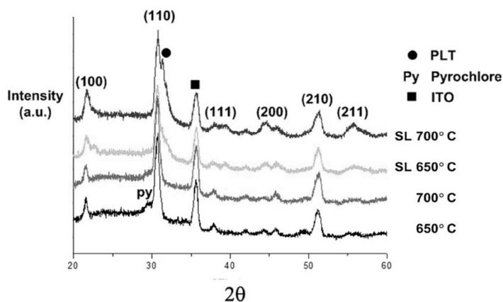
**Fig. 3.** XRD patterns of the PLZT (08/65/35) films without and with PLT seeding layer prepared with annealing time of 30 min.
