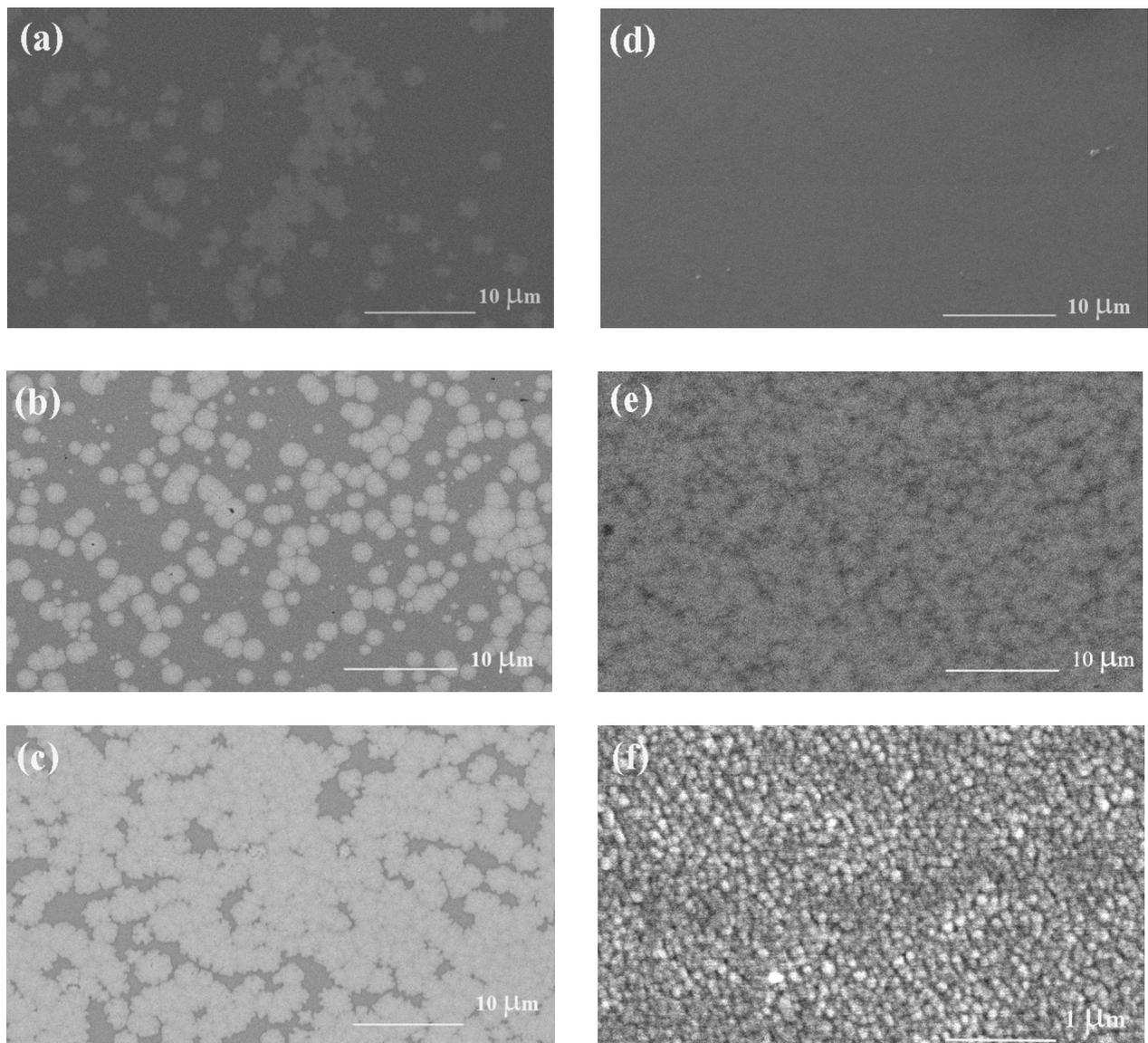
**Fig. 2.** SEM photographs of the PLZT films (a-c) without and (d-f) with the PLT seeding layer annealed at (a,d) 600°C, (b,e) 650°C and (c,f) 700°C, 30 min.
