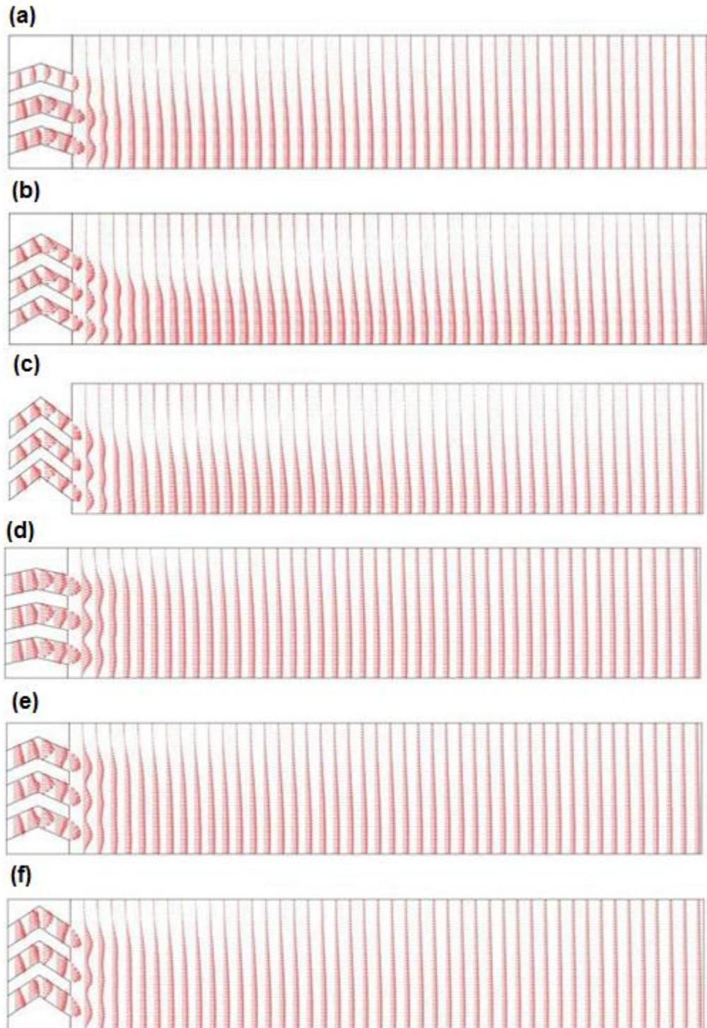
**Fig .6.** Velocity vector within concrete block and room with different blocks.
