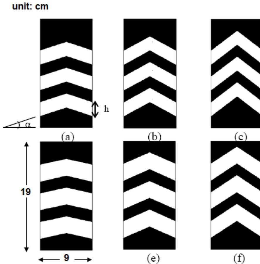
Fig. 3. Schematic of a new prototype of concrete block [12].
