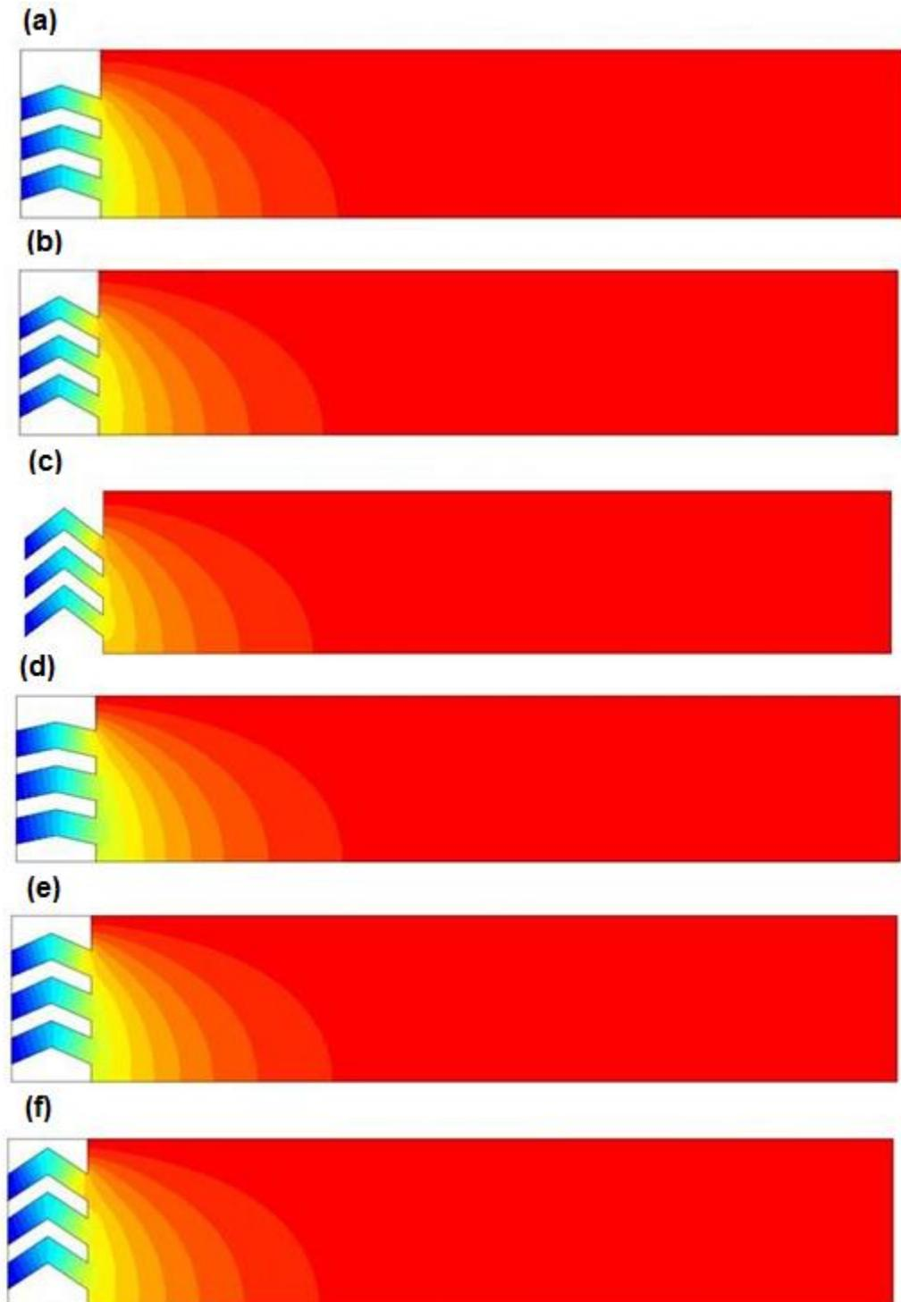
**Fig .7.** Temperature contour within concrete block and room with different blocks.
