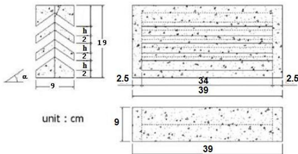
**Fig .1.** Dimensions of the vented concrete block with reverse V-shape ( $\Lambda$ ) opening [3].
