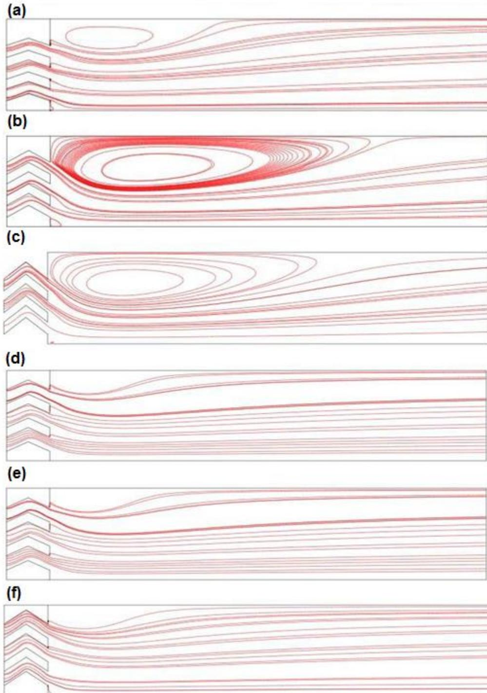
**Fig. 5.** Streamlines within concrete block and room with different blocks.
