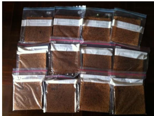
Fig.1. Binderless particleboard from durian peel [1].
