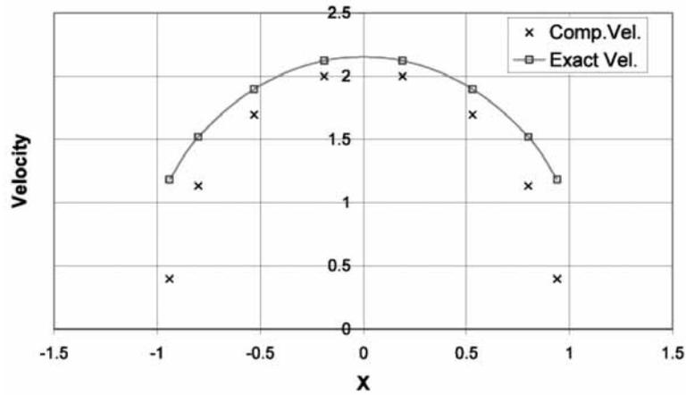
**Fig. 4.** Comparison of exact and computed values over the boundary of a circular cylinder for 16 constant boundary elements.
