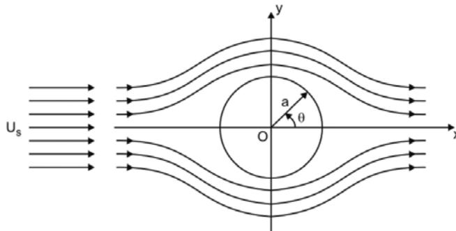
**Fig. 1.** Oseen's flow around a circular cylinder.
