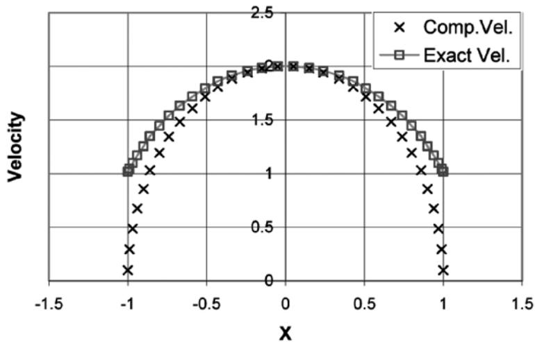
**Fig. 6.** Comparison of exact and computed values over the boundary of a circular cylinder for 64 constant boundary elements.
