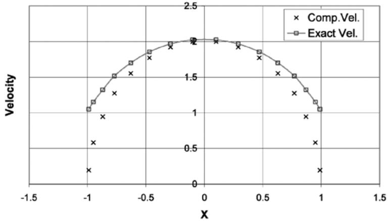
**Fig. 5.** Comparison of exact and computed values over the boundary of a circular cylinder for 32 constant boundary elements.
