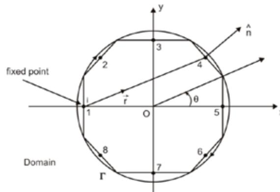
**Fig. 2** The discretization of the surface of a circular cylinder into constant boundary elements
