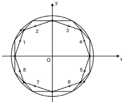
**Fig. 3** Discretization of constant boundary elements.
