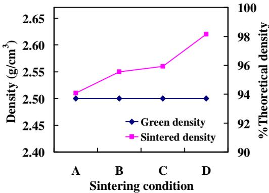
Fig. 3 Variations of sintering conditions on the sintered density of Alumix 231.
