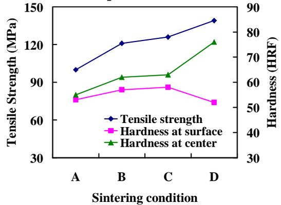
Fig. 5 Tensile strength and hardness tested at the surface and centre of the specimens sintered in various conditions.
