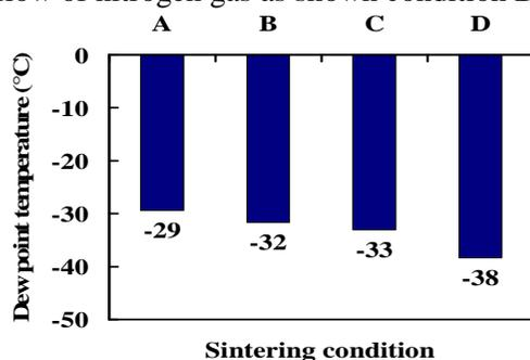
**Fig. 2** Furnace dew point temperatures of the nitrogen atmosphere corresponding to the various sintering conditions.
