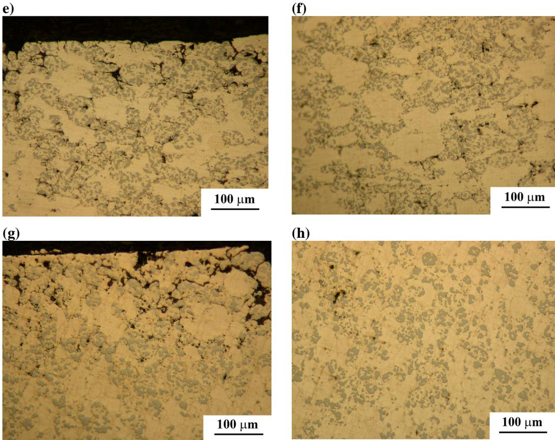
**Fig. 6** Microstructural images of Alumix 231 specimens sintered in various conditions; condition A (a) and (b), condition B (c) and (d), condition C (e) and (f), and condition D (g) and (h). The left images show the microstructure at the area near the specimen surface, while the right images show the microstructure at the centre of specimens.
