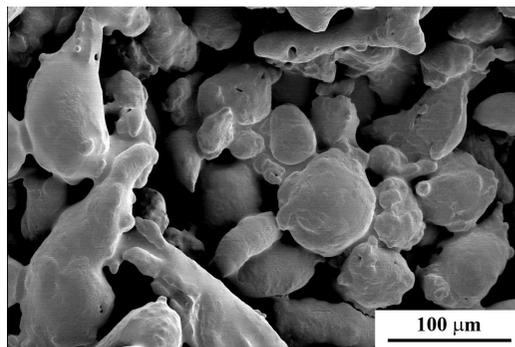
**Fig. 1** Scanning electron image of Alumix 231 powder.
