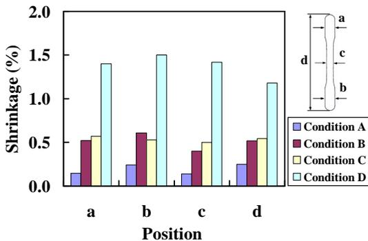
Fig. 4 Shrinkage of the sintered specimens from their green dimension.
