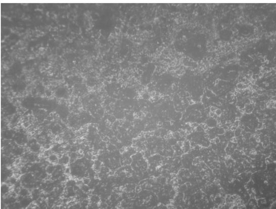
**Figure 6** Microstructure on the Weld Zone (WZ) for the heat input per unit length of 0.188 kJ/mm
