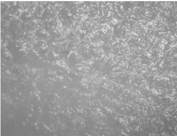
**Figure 5** Microstructure on the Heat affected Zone (HAZ) region for the Heat input per unit length of 0.188 kJ/mm
