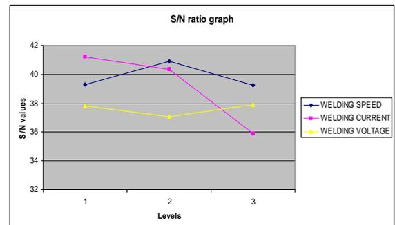
**Figure 2** S/N Ratio Graph for Dissimilar Metals Welding
