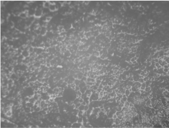
**Figure 4** Microstructure on the Base Metal (BM) region for the heat input per unit length of 0.188 kJ/mm
