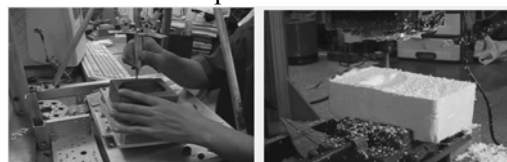
The master arm with force reflection The Slave arm (5-axis) Figure 27 Master-Slave Arm Haptic device
