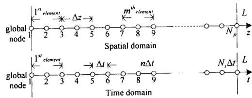
**Fig.2** Subdividing into line elements in the spatial domain and time domain.
