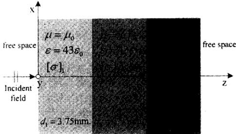
**Fig.4** Three-layer anisotropic media
