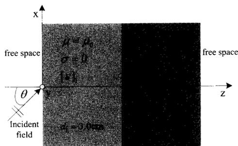
Fig.3 Two-layer anisotropic media
