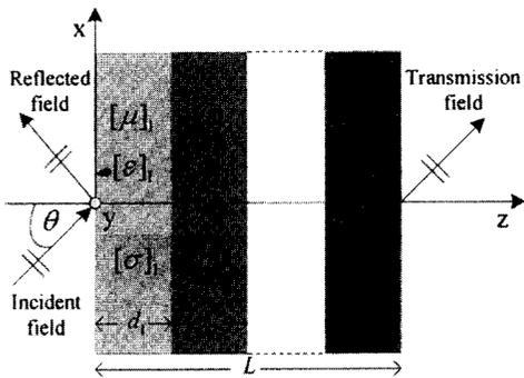
**Fig.1** Geometry of multi-layered anisotropic media with a obliquely incident plane wave.
