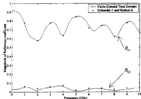
**Fig.6** Magnitude of reflection coefficient  $R_{11}$  and  $R_{12}$  based on Fig.4 (solid line for FETD and asterisk for FDTD by Schneider and Hudson).
