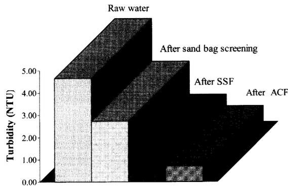
**Fig. 3** Decrease of turbidity at various steps of unit processes
