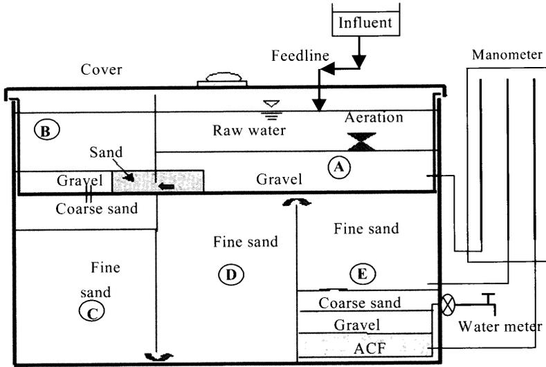
Fig. 1 Schematic diagram of the household water filter
