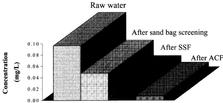
**Fig. 5** Decrease of iron at various steps of unit processes
