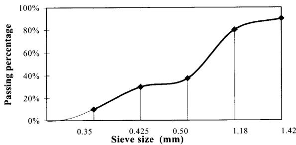
Fig.2 Sieving curve of filter medium
