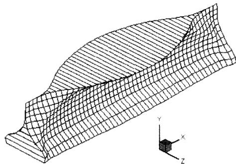
**Figure. 7** Optimum design of a simply-supported beam subjected to a horizontally-translated vertical load.
