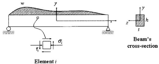
**Figure. 2** A simply supported beam under distributed load.
