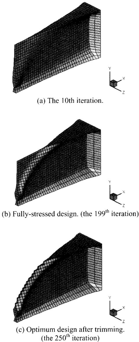
**Figure. 5** Shapes of the short cantilever beams. (z-scale is magnified three time)
