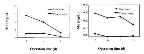
Figure 5 Variation of manganese in effluent
