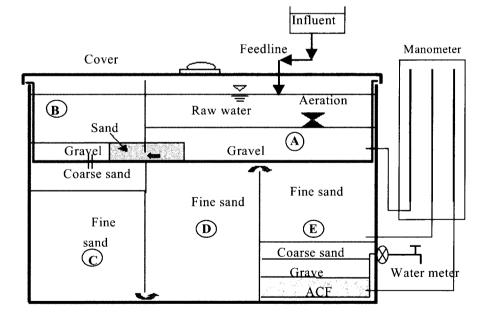
Figure 1 Schematic diagram of the household water filter
