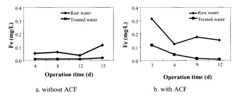
Figure 4 Variation of iron in effluent
