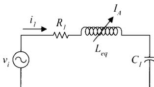
**Fig.5** Series RLC resonance circuit
