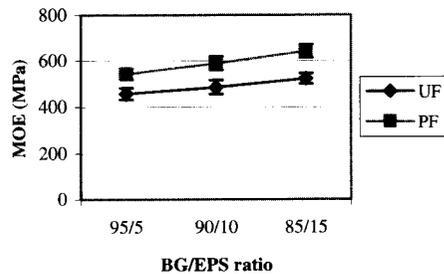
**Figure 8** MOE (Modulus of Elasticity) vs BG/EPS ratios
