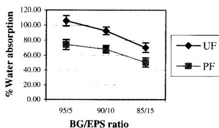
**Figure 3** % Water absorption vs BG/EPS ratios
