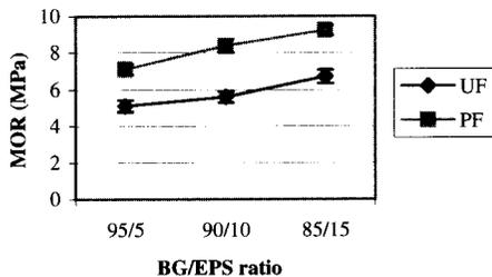
**Figure 5** MOR (Modulus of Rupture) vs BG/EPS ratios
