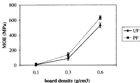
**Figure 12** MOE (Modulus of Elasticity) vs board densities
