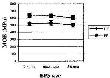
**Figure 10** MOE (Modulus of Elasticity) vs EPS sizes
