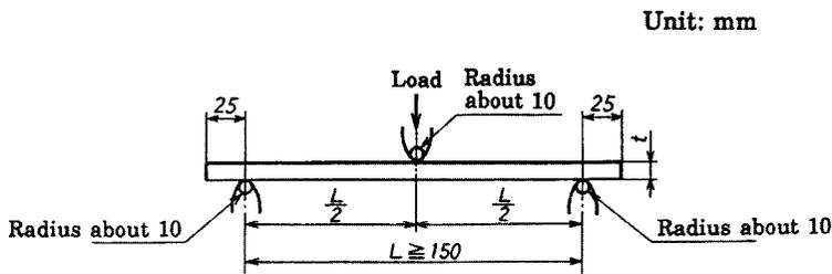
Figure 2 Test apparatus for bending strength
