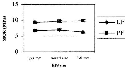
**Figure 9** MOR (Modulus of Rupture) vs EPS sizes
