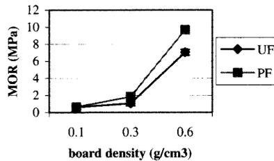
**Figure 11** MOR (Modulus of Rupture) vs board densities
