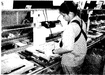
Figure 6. 1 st conveyor section (panel assembly process)
