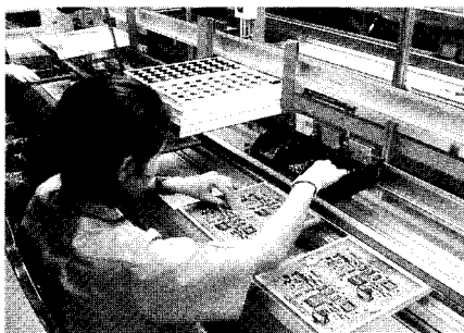
Figure 2. 1 st conveyor section (material insertion process)
