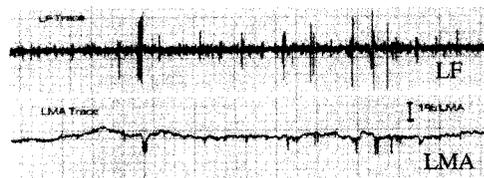
Figure 3 LF and LMA signals of wire rope
