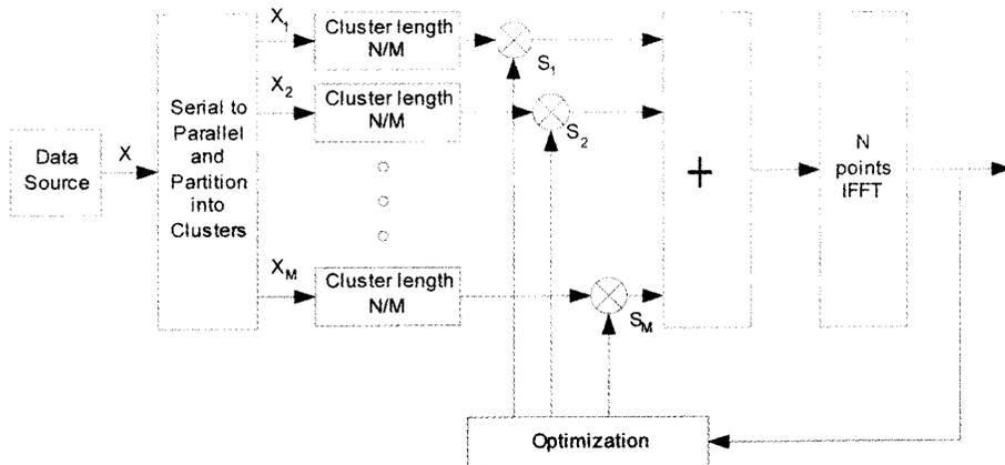
**Figure 4:** Block Diagram for envelope scaling
