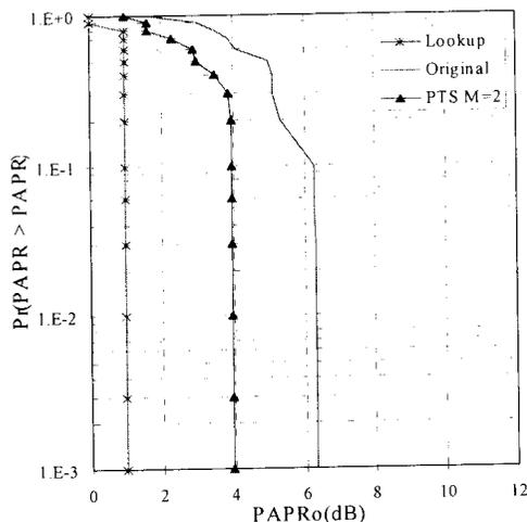
**Figure 3:** Comparison of CCDF of PAPR with lookup table and PTS with  $M = 2$
