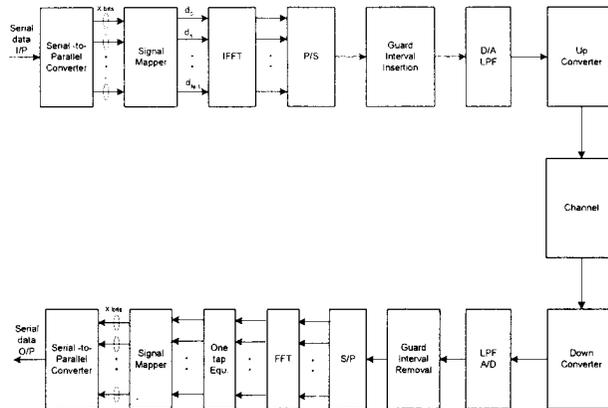
**Figure 1:** Basic FFT based OFDM system
