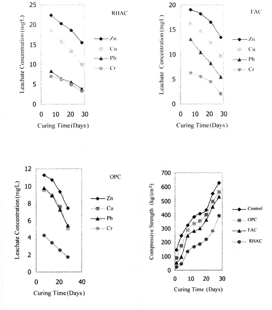
**Figure 4.** Effect of Curing Time on Leachate Concentration and Compressive Strength.
