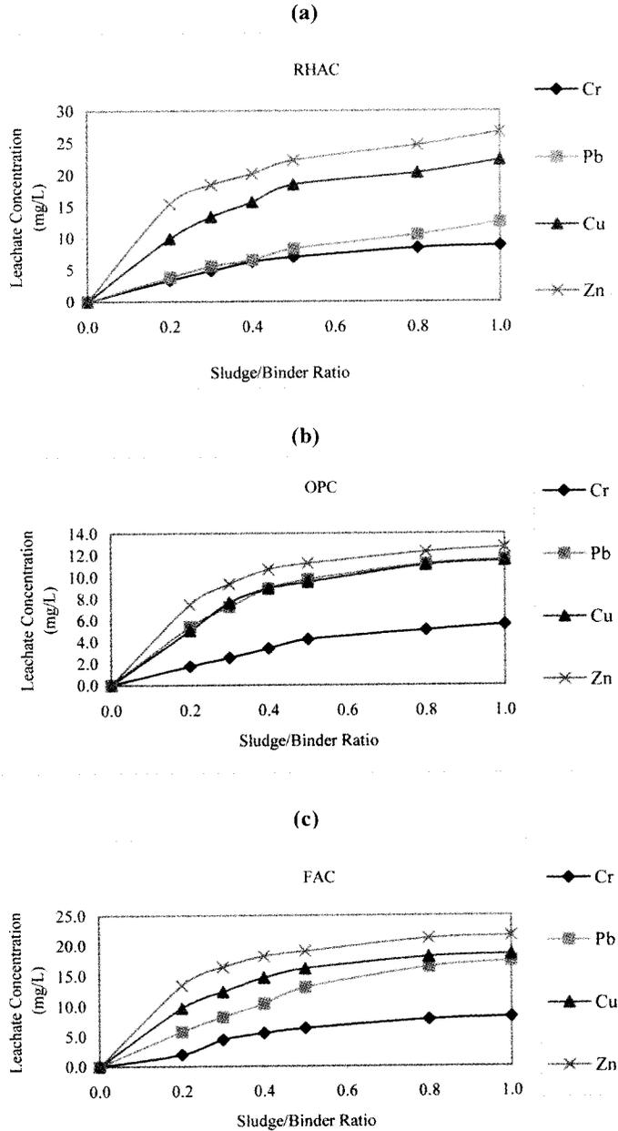
**Figure 3.** Effect of Sludge/Binder Ratio on Leachate Concentration for (a) RHAC, (b) OPC, and (c) FAC Binders.
