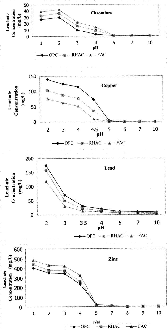
Figure 5. pH Dependent of Leaching Behavior for Cr, Cu, Pb and Zn.
