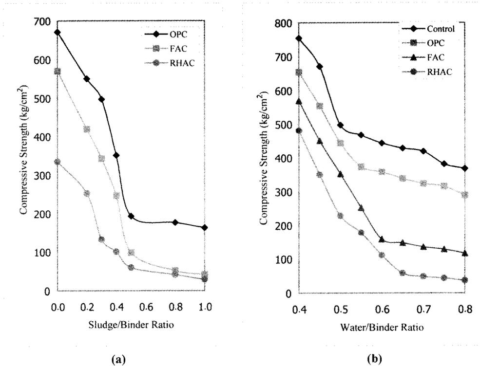
**Figure 2.** Effect of (a) Sludge/Binder and (b) Water/Binder Ratios on Compressive Strength for OPC, FAC and RHAC Binders.
