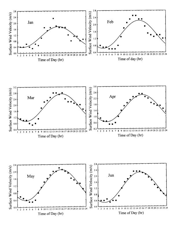
Fig. 1 (a) Hourly mean surface wind velocity (January-June)
