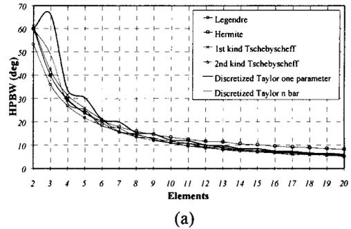
Fig.4 (a) Half power beamwidth for various number of elements (b) Half power beamwidth for various side lobe ratios
