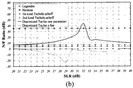
**Fig.6** (a) The nearest to the furthest minor lobe ratio for various number of elements (b) The nearest to the furthest minor lobe ratio for various side lobe ratios
