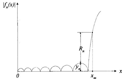
**Fig. 1** How to form the main beam and the minor lobes
