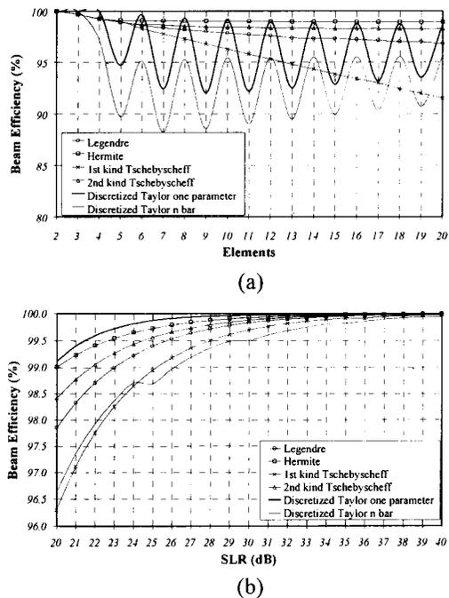
Fig.8 (a) Beam efficiency for various number of elements (b) Beam efficiency for various side lobe ratios
