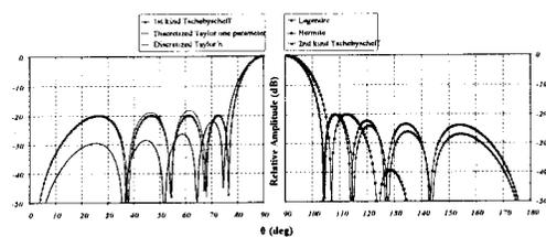
**Fig. 2** Radiation pattern of six arrays
