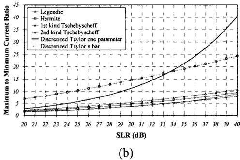
Fig.3 (a) Maximum to minimum current ratio for various number of elements (b) Maximum to minimum current ratio for various side lobe ratios
