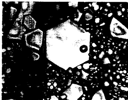
Fig. 1. Hexagonal Crystallites in M-Type Barium Ferrites Doped with Bismuth Oxides. ( x 1000 )
