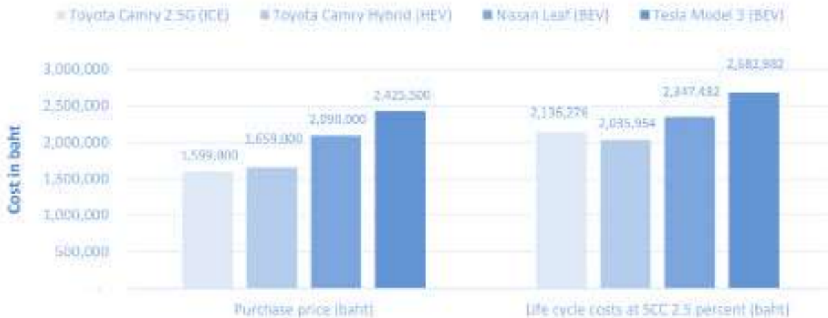
Figure 11: Life cycle cost of Toyota Camry vs. Nissan LEAF (BEV) vs. Tesla Model 3 (BEV) at 3,100 km/month
