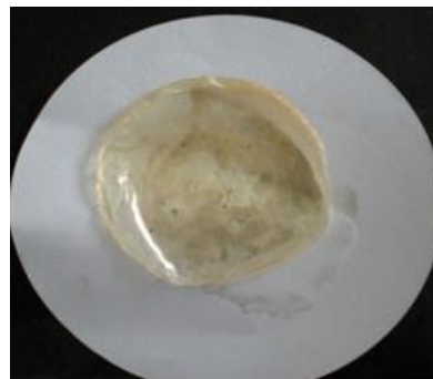
Figure 1 Aceclofenac transdermal patch prepared by solvent casting
