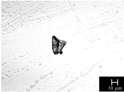
Fig. 1 Mild sliding wear debris
