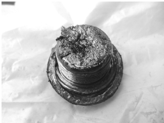
Fig. 9 Condition of a MCD located in the final drive after 10,000 km
