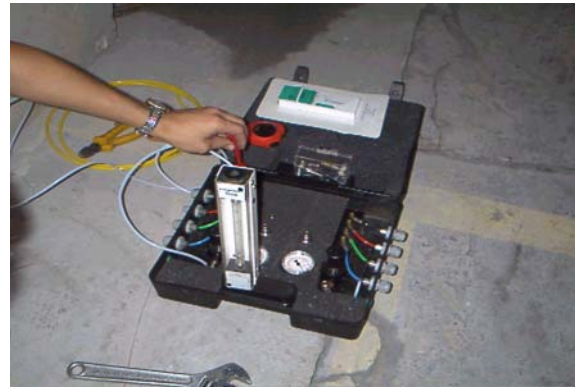
Figure 5 The air purity tester was used to measure the mixture of air
