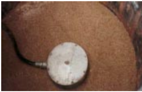
Figure 11 Pressure cell was installed beneath treated embankment
