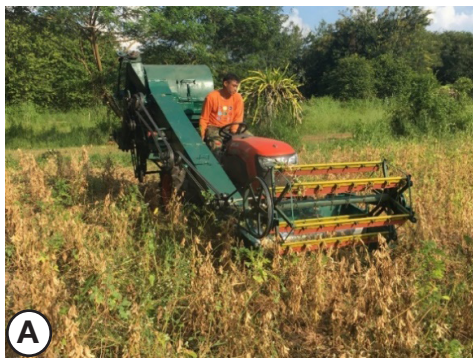
Figure 7 Performance test evaluation of soybean combine harvester in the field (A) row planting (B) board planting
