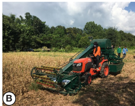
Figure 7 Performance test evaluation of soybean combine harvester in the field (A) row planting (B) board planting
