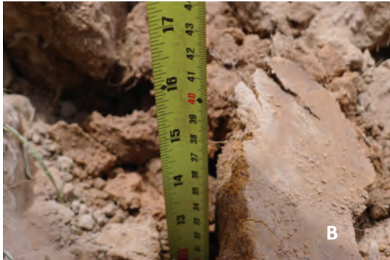
Figure 4 Prototype I test (A) and working depth of prototype I (B)
