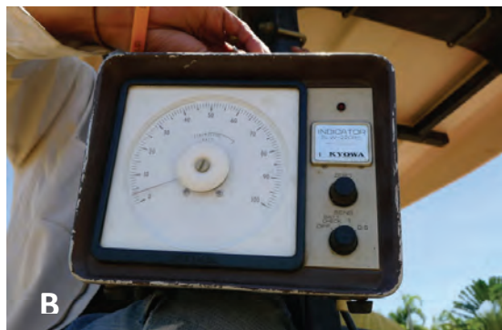
Figure 4 Measuring of Draft for a tractor mounted implement (A) and indicator Kyowa (B)
