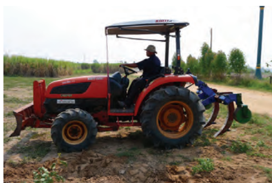
Figure 7 Testing the subsoiler attached to tractor 50 hp in sugarcane field
