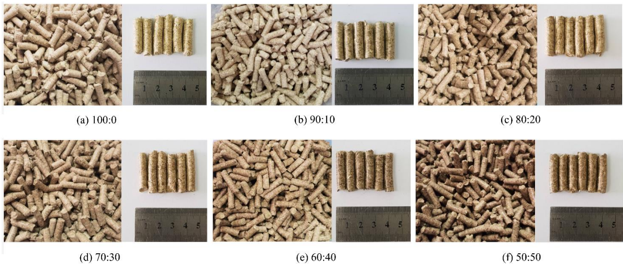
Figure 2 Effect of mixing ratios on physical appearance of leucaena pellets (a) 100:0, (b) 90:10, (c) 80:20, (d) 70:30, (e) 60:40, and (f) 50:50
